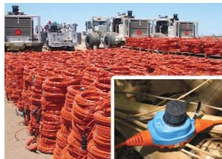
Figure 1. Global's Belridge crew operating 13,500 channels of Sercel 428XL equipment. (All photos courtesy of Global Geophysical)
