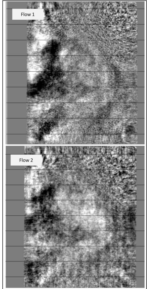
Figure 3b: Timeslice displays with flow 1 (cascading velocity filter and deburst) and with flow 2 (random noise attenuation). A strong footprint is readily apparent on the random noise attenuation flow and alters the processing decision which may have been made from inspection of shot records and/or inline stacks.
