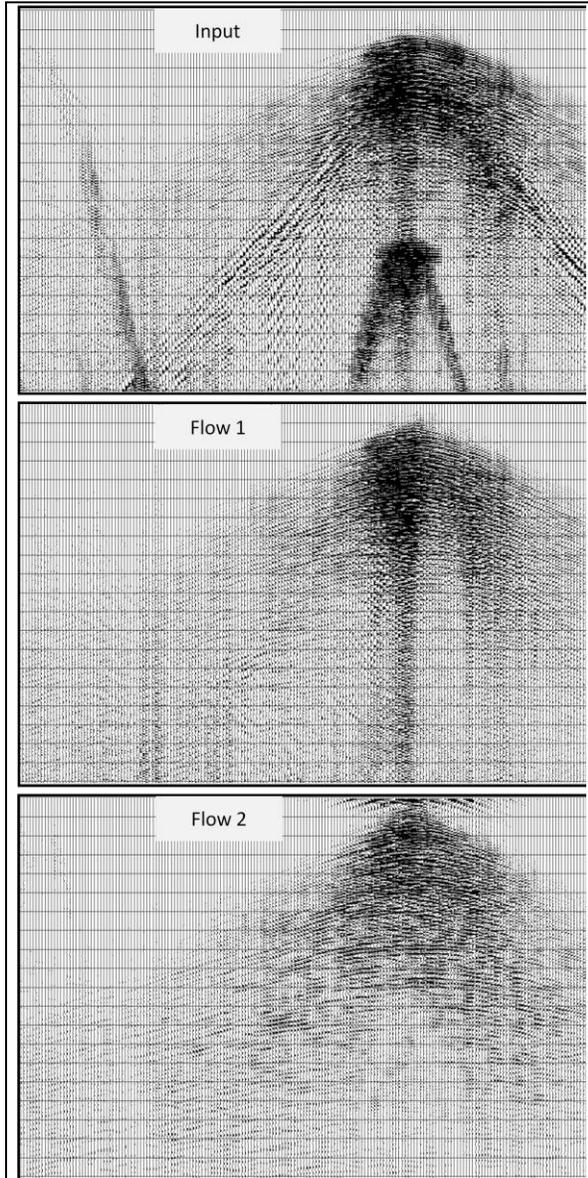
Figure 3a: Shot records before noise attenuation, with flow 1 (cascading velocity filter and deburst), and with flow 2 (random noise attenuation). The random noise attenuation flow appears to have removed more noise and the events are more continuous.
