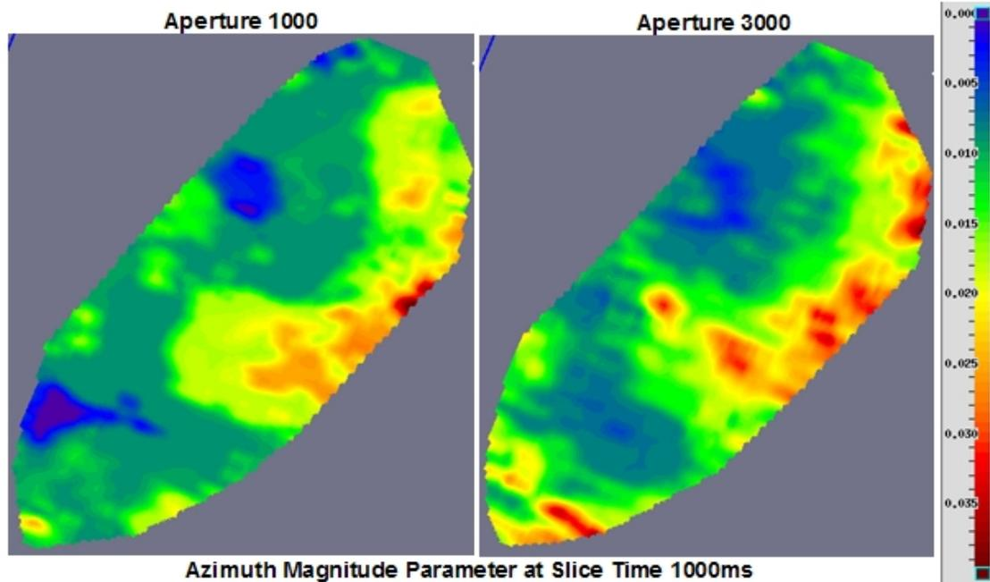
Figure 6: Azimuth parameter computation using 2 different apertures in the migration analysis. Comparison of the 1000 foot aperture result to the 3000 foot aperture results at time slice 1000 ms. The depth to the horizon is 6000 feet.
