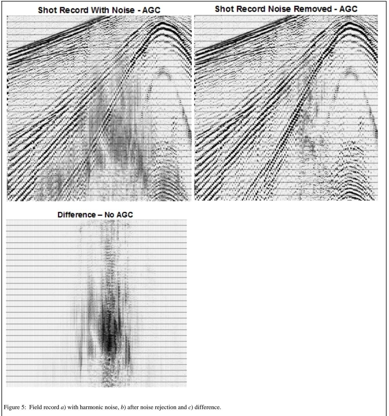
Figure 5: Field record *a*) with harmonic noise, *b*) after noise rejection and *c*) difference.
