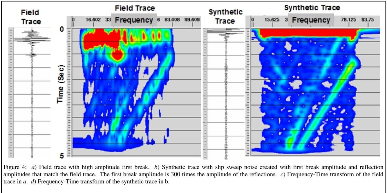
Figure 4: a) Field trace with high amplitude first break. b) Synthetic trace with slip sweep noise created with first break amplitude and reflection amplitudes that match the field trace. The first break amplitude is 300 times the amplitude of the reflections. c) Frequency-Time transform of the field trace in a. d) Frequency-Time transform of the synthetic trace in b.
