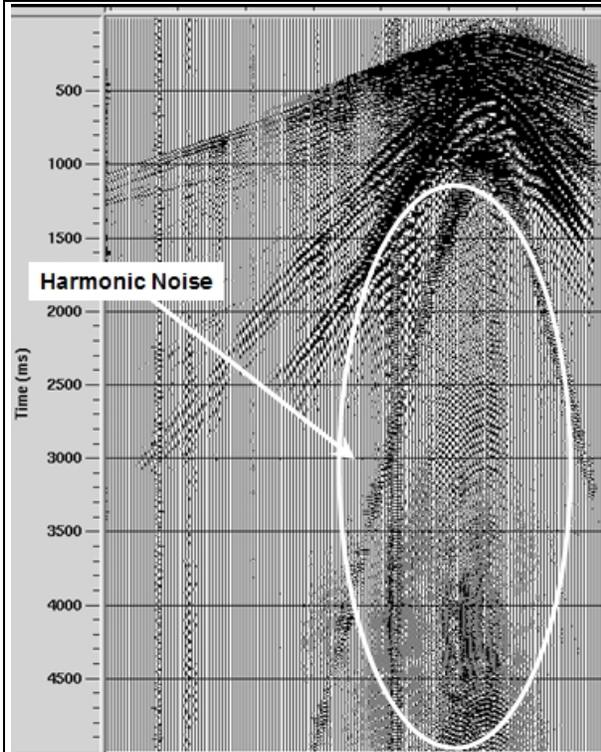
Figure 1: Example of harmonic noise on the correlated traces of a field record.
