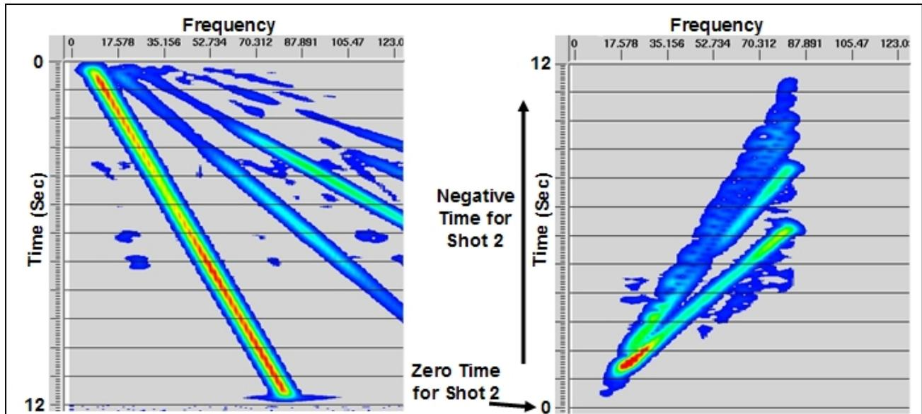
Figure 3: a) Frequency-Time transform of the Ground Force signal from Figure 2. b) FT transform of derived filter. This is the harmonic noise filter used to estimate harmonic noise in prior shot.
