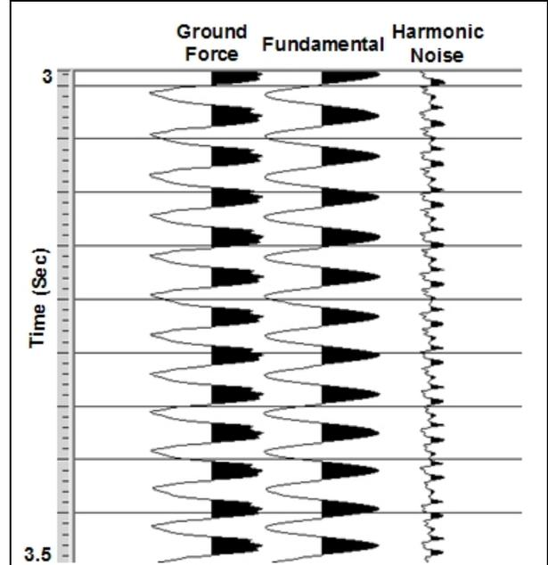
Figure 2: Example of a Ground Force recording, the separated fundamental, and the separated harmonic noise for the time window 3.0 to 3.5 seconds.
