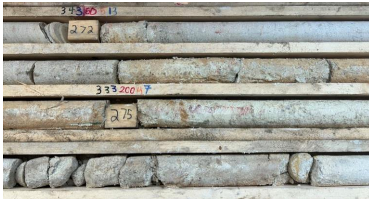
Altered sandstone 12 to 20 metres above the unconformity in Target Area B (LE24-181, 271.8- 276.7m). The core is strongly bleached with intervals of desilicification and strong clay alteration
